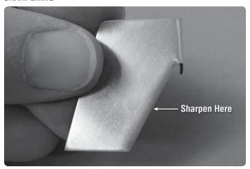
It's best to sharpen the turn fin to a razor-sharp edge. This will eliminate drag and reduce lift. Remember as a rule of thumb, if it touches the water, it needs to be sharp or have sharp edges. GRIMRACER SAYS! Sharpen the outer edge of the turn fin toward the inside of the boat. This is a great way to help control prop torque.
