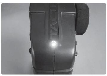
Turn the transmitter on by pressing the "Power" button on the right side of the transmitter. The battery indicator light (LED) should glow green. If the light is flashing, the batteries are low and need to be replaced.
