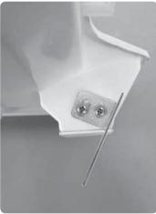
The turn can be adjusted to a vertical setting or for more aggressive steering tucked under the boat. It's important to note that this boat does not require much tuck-under. The boat runs very well with the fin vertical.
