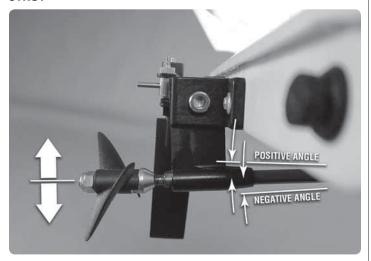
The strut can be *tweaked* to change the ride of the boat but only experienced modelers should attempt this. If you are going to *tweak* the strut, remove the prop shaft and prop. Loosen the strut bolt. Move or adjust the strut, taking care not to lose the alignment of the driveshaft to the motor coupler. If needed, you might have to re-bend this area to regain alignment.
