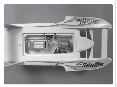
In your boat you will find a length of hook and loop on the battery tray. Remove the piece of hook and loop and install onto the battery back. Install the battery into the boat like shown in the picture.
