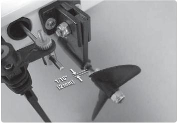
Leave about a 1/16" [2mm] gap between the front of the drive dog and the back of the brass tube. Retighten the shaft coupler screws.
