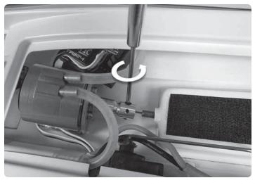
Using a 2mm hex wrench, loosen the screws holding the drive cable to the motor coupler. It is important to note that there are two set screws holding the shaft in position.
