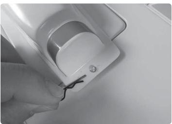
Turn on your transmitter. Remove the main canopy by pulling the pin on the back of the cowl.
