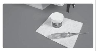
It is important to remove and re-lubricate the driveshaft after running for the day. Make sure the battery pack is unplugged. You will need a 2mm hex wrench, GrimRacer Cable Grease and some paper towels.
