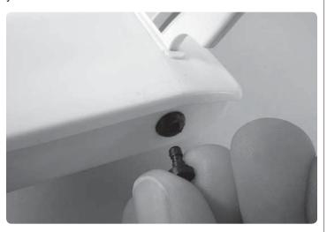
**IMPORTANT:** If your boat takes on a large amount of water and stalls, don't worry. **Foam flotation will keep it from sinking.** You will have to retrieve the boat and remove the canopy to release any water that might have entered. If the inside is flooded, remove the transom plug from the back of the boat and let the water drain. Allow the boat to fully dry before operating it again. Remember to re-install the transom plug before running.
