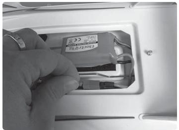
Tuck the wires neatly under the decking.
