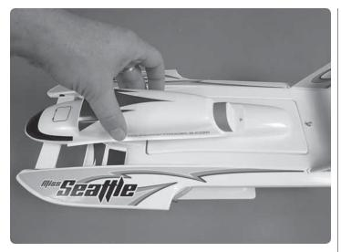
Lightly lift the back and carefully slide the cowl forward.
